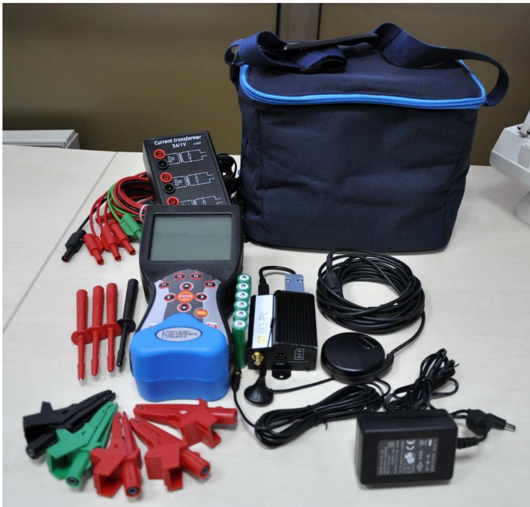
Fig. 3. STER PMU complete measurement set
