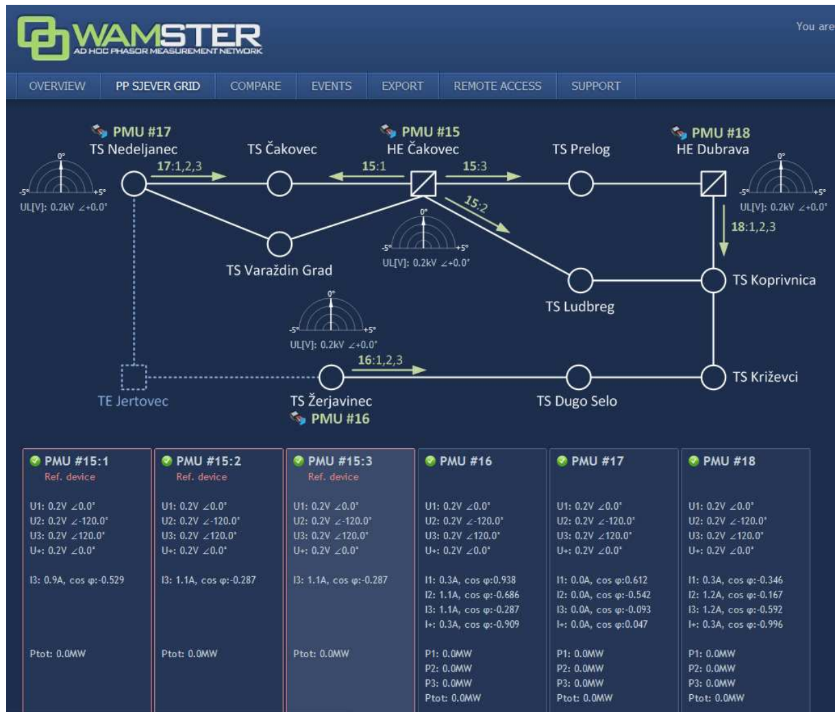
Fig. 17. dedicated WAMSTER – custom single line diagram: voltage, current and power information
