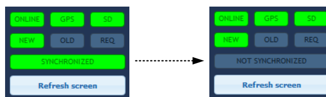
Figure 6.27: If the remote instrument is in a different menu than the one shown on the web page, remote status will change to "NOT SYNCHRONIZED"
