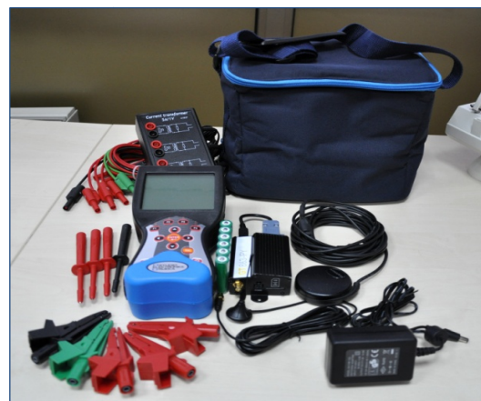
Fig. 1. STER PMU with all accessories. Only a single power supply adapter is needed.
