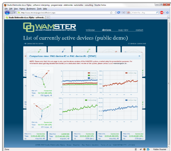
Fig. 4. Synchronized comparison of two PMU devices, in real time
