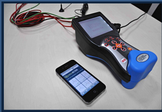
STER PMU is a handheld, portable synchrophasor, power quality meter and continuous data recorder.
