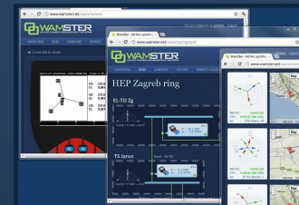
Online user interface is used for status monitoring, data analysis, export and remote device setup.
