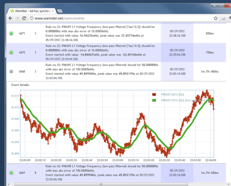
Triggers are configured on various quantities. Events are easily analyzed using the web interface
