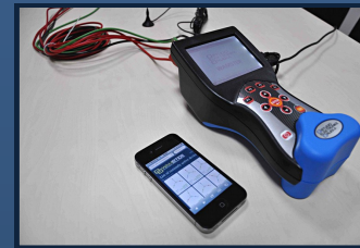
STER PMU is a small, handheld portable synchrophasor device.
