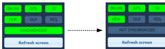
Figure 5.27: If the remote instrument is in a different menu than the one shown on the web page, remote status will change to "NOT SYNCHRONIZED"
