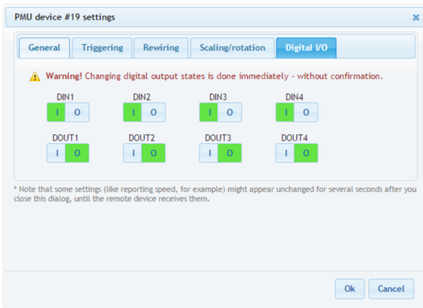
Figure 5.9: Digital inputs and outputs can be controlled using the last tab
