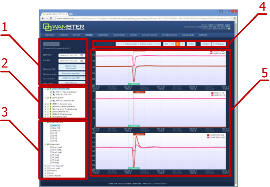
Figure 5.18: Trends page can be used to view and compare measurements during different time periods
