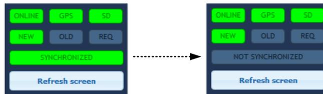
Figure 4.27: If the remote instrument is in a different menu than the one shown on the web page, remote status will change to "NOT SYNCHRONIZED"
