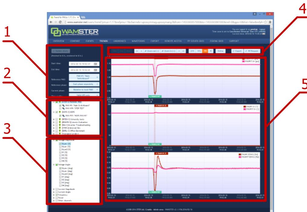
Figure 4.18: Trends page can be used to view and compare measurements during different time periods
