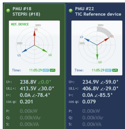
Figure 4.11: Device selected as the reference device (left), and a different device with relatively rotated synchrophasors (right)
